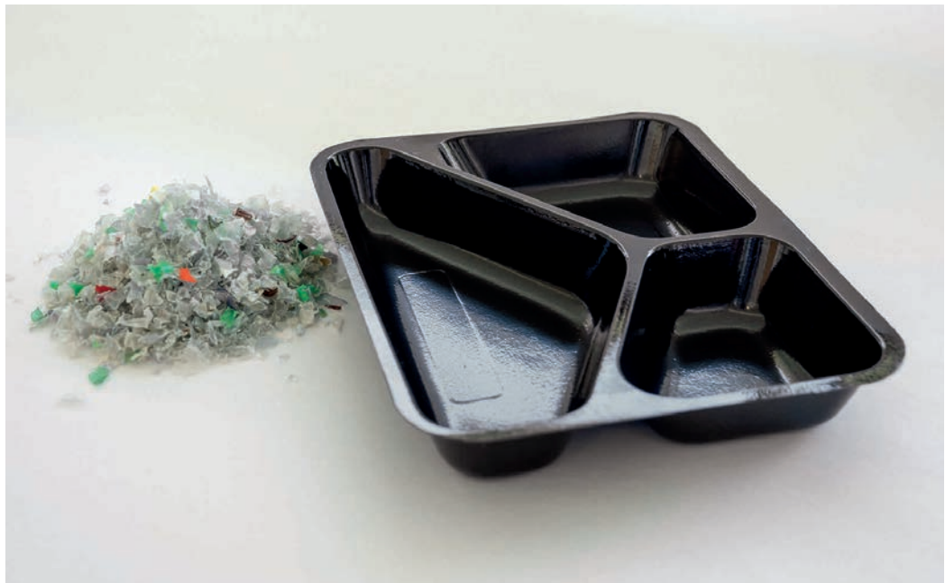
Thermally stable rCPET food trays made from multicolor APET bottle flakes (© Illig)
