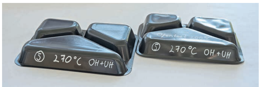
Fig. 7. rCPET food trays made from material sheet 5 before and after the oven test at 270°C on upper and lower heater (© Illig)
