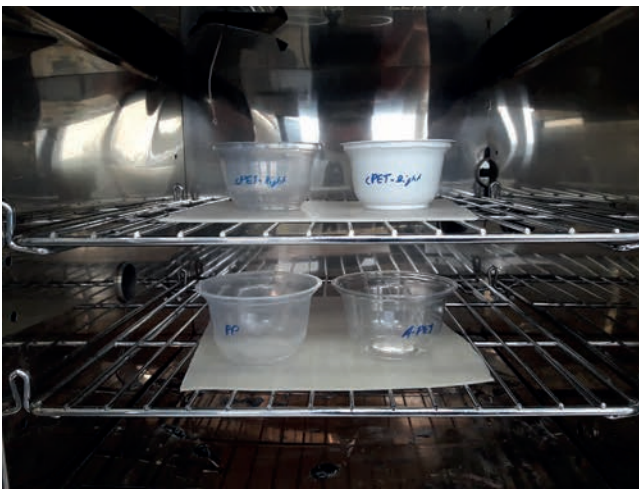
Fig. 5. Comparison of the tested samples before and 30 min after the oven test at 100 °C © Illig
