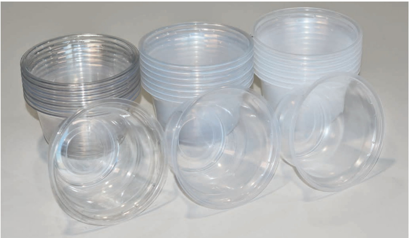
Quite transparent: three materials competed against each other in a practical test. APET on the left, CPET-light in the middle and PP on the right © Illig
